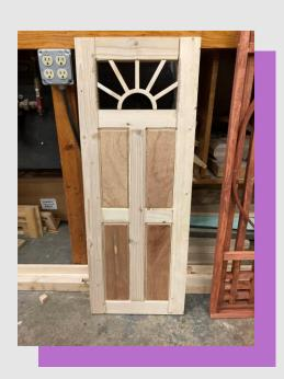
Using tongue and grooves that were ¾" was the best joining technique not only to have clean and strong connections, but to also allow for ¾" plywood to be slotted into the grooves to begin the inside panel inset. The top opening was filled with a piece of acrylic, spaced out to fit the groove perfectly, leaving the window flush with the plywood panels.
